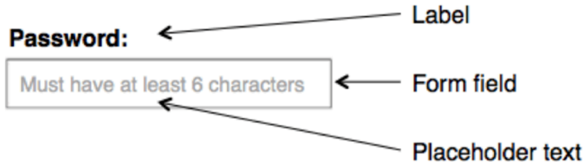
Figure 14: image showing examples of what is a label, a form field and a placeholder text.
